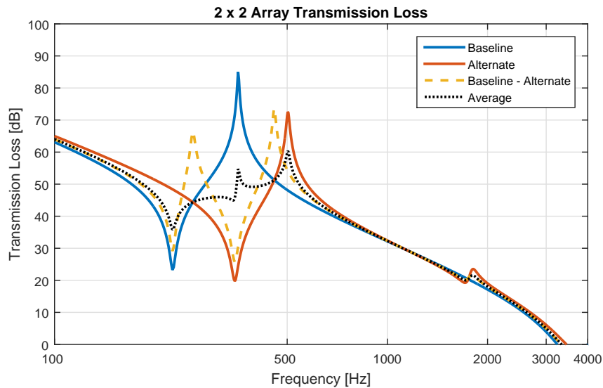
Figure 5.24: Transmission loss of baffled multi-cellular arrays with different unit cells. Baseline (blue solid), Alternate (red solid), combined (dashed)
